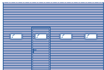
Sectional door APU F42 with wicket door with trip-free threshold
