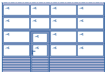
Sectional door APU F42 with wicket door with trip-free threshold
