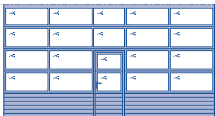
Sectional door APU F42 with wicket door with trip-free threshold
